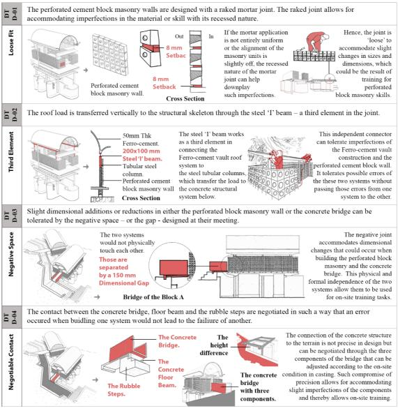
Figure 2: Building example - tolerance by detail
