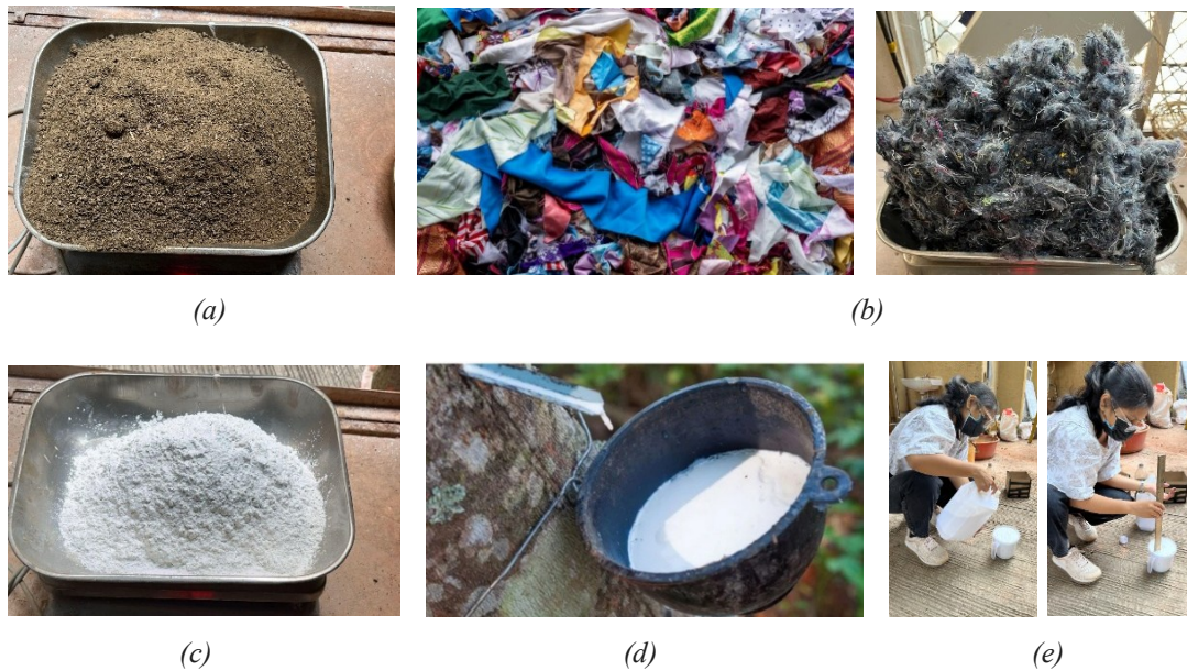
Figure 7: (a) cow dung powder; (b) textile waste; (c) lime powder; (d) Natural Rubber Latex (NRL); (e) Natural Rubber Latex (NRL) mixed with water
